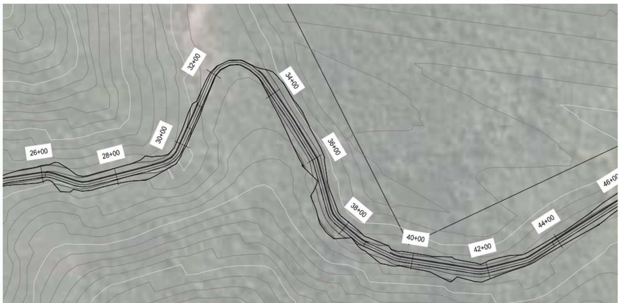
Figure 4 - Example Corridor Plan View with Cut and Fill Sections in AutoCAD Software
