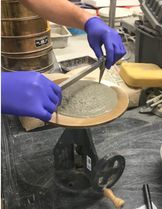
Figure 4.4: Measuring mortar workability according to ASTM C 1437
