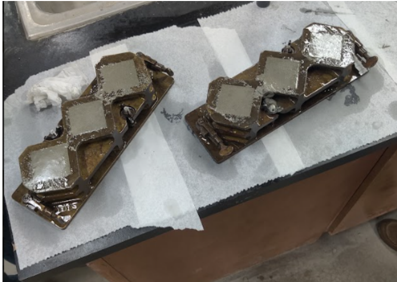
Figure 4.5: Mortar that passed the water retention test put into the molds according to ASTM C 1437
