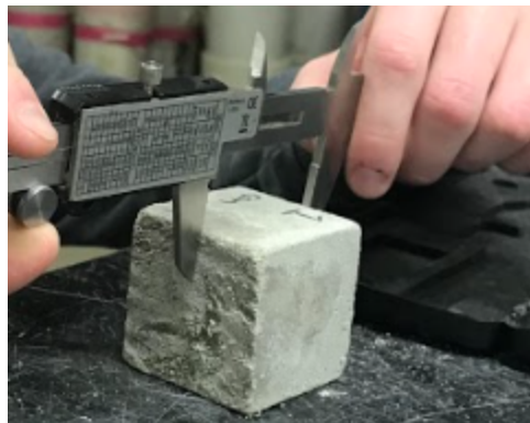
Figure 4.6: Team member measuring the area of the cube face.
