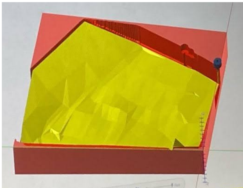
Figure 9. CNC router model of streambed
