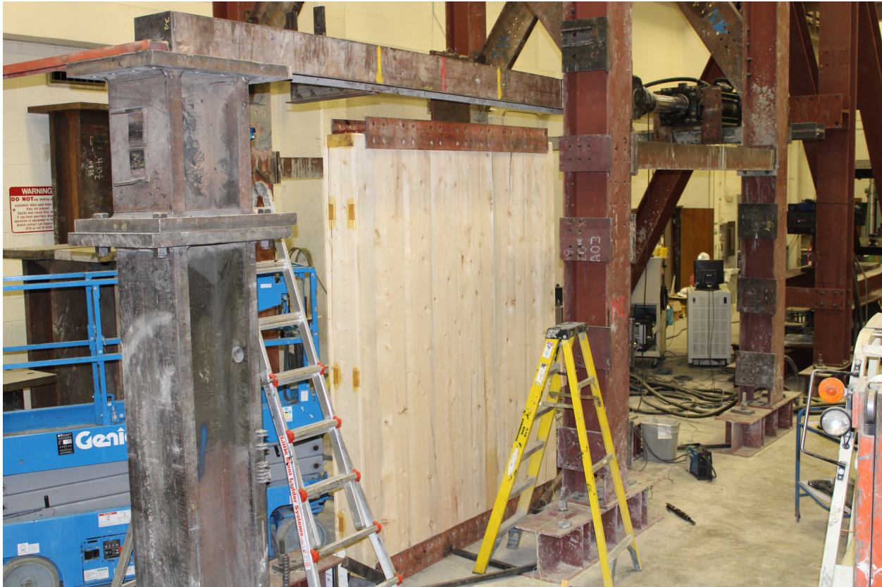
Figure 2: Preliminary Testing Frame Design
