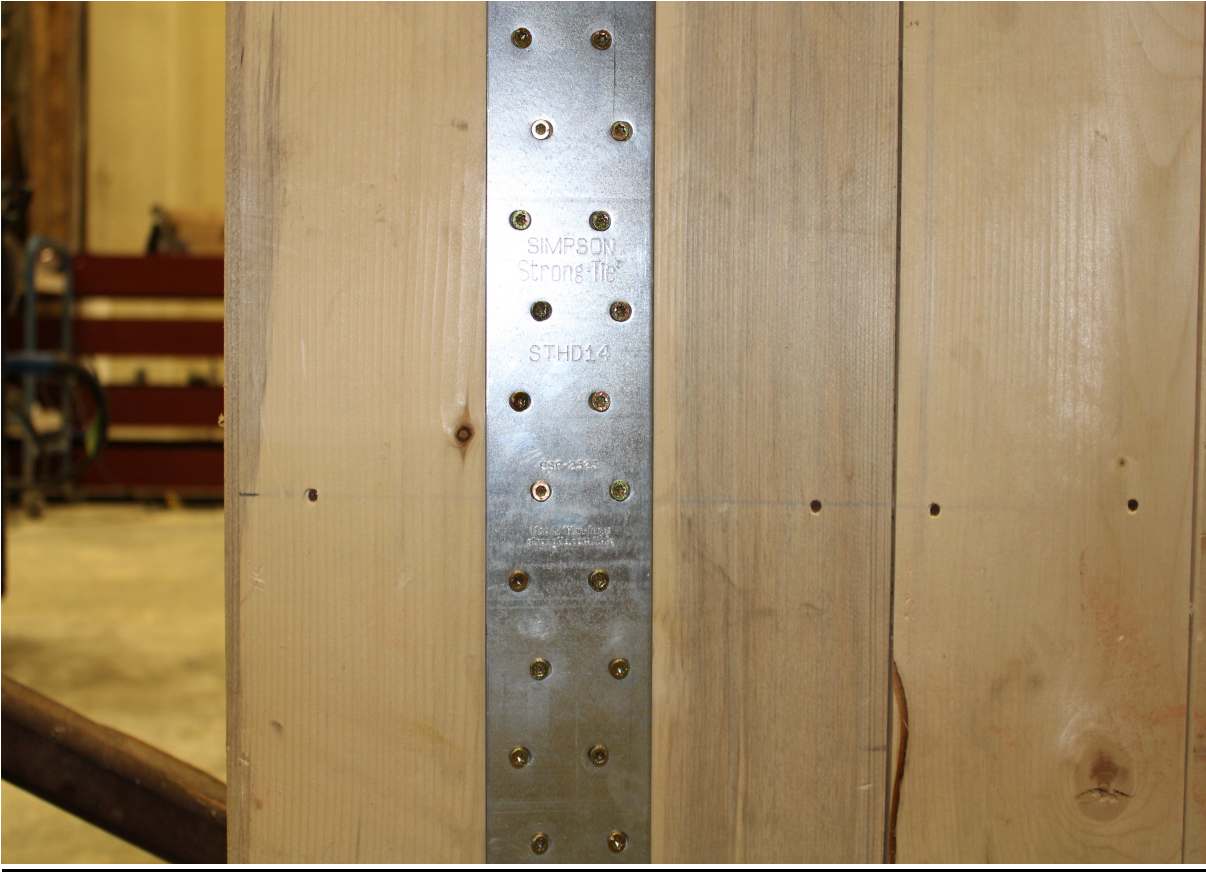
Figure 14: Wall 4 STHD14 Straps
