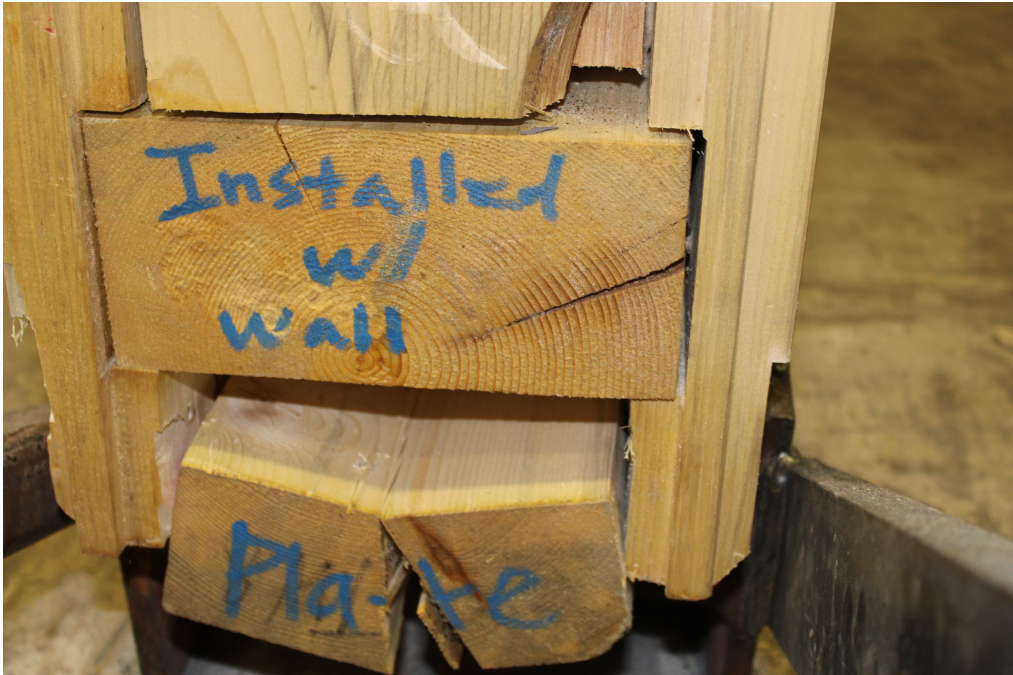
Figure 13: Third Wall Secondary Failure Mode
