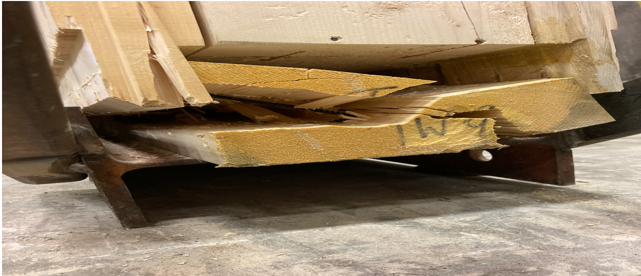
Figure 9: Wall 2 Failure Mode
