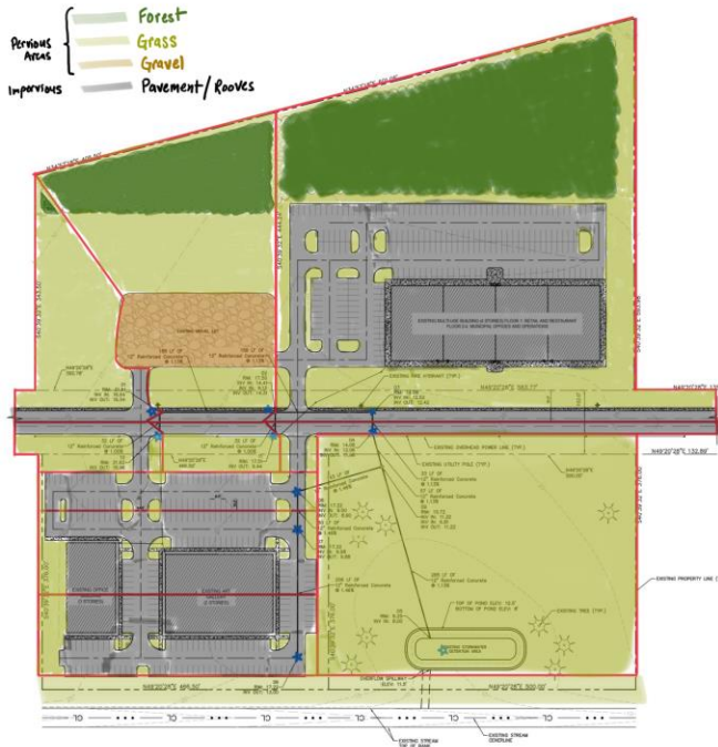
Figure C-1. Pre-improved Pervious and Impervious Areas
