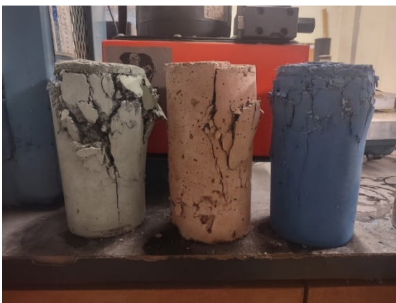
Figure 4: Lime concentrations of 10%, 15%, and 20% (left to right).
