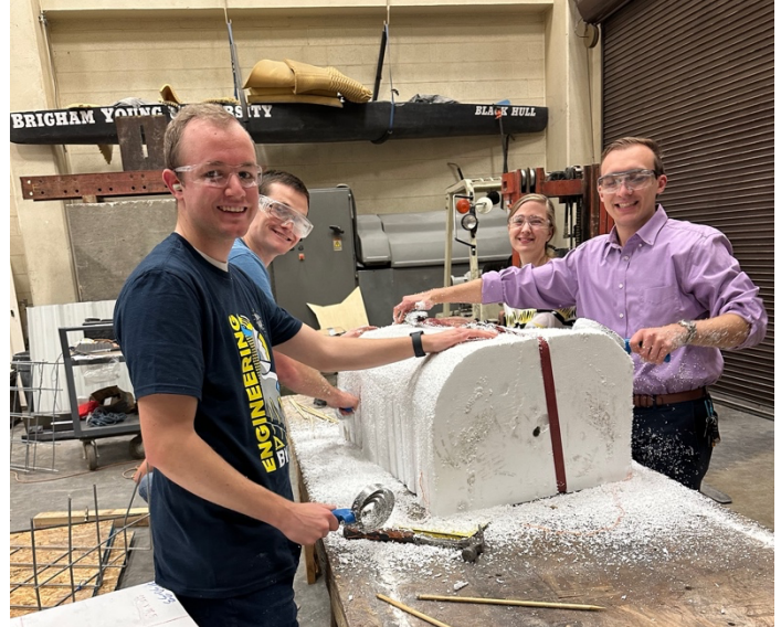
Figure 6: Rebar enforced form shaping with curry comb.
