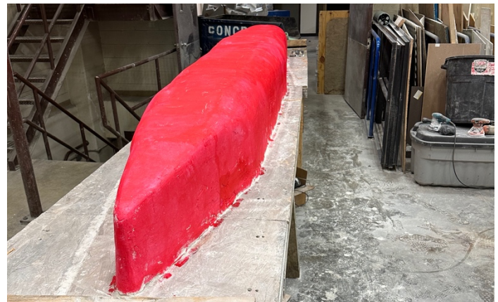
Figure 7: RedGuard sealant on canoe form.
