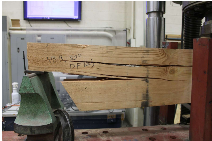
Figure 9 - Example of Significant Shear Failure
