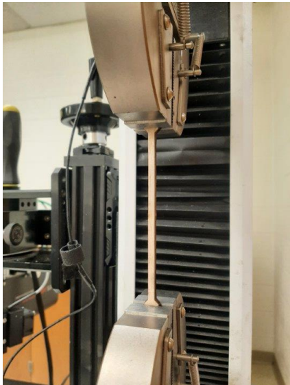
Figure 2: Tensile and Compression Test to Determine Modulus of Elasticity
