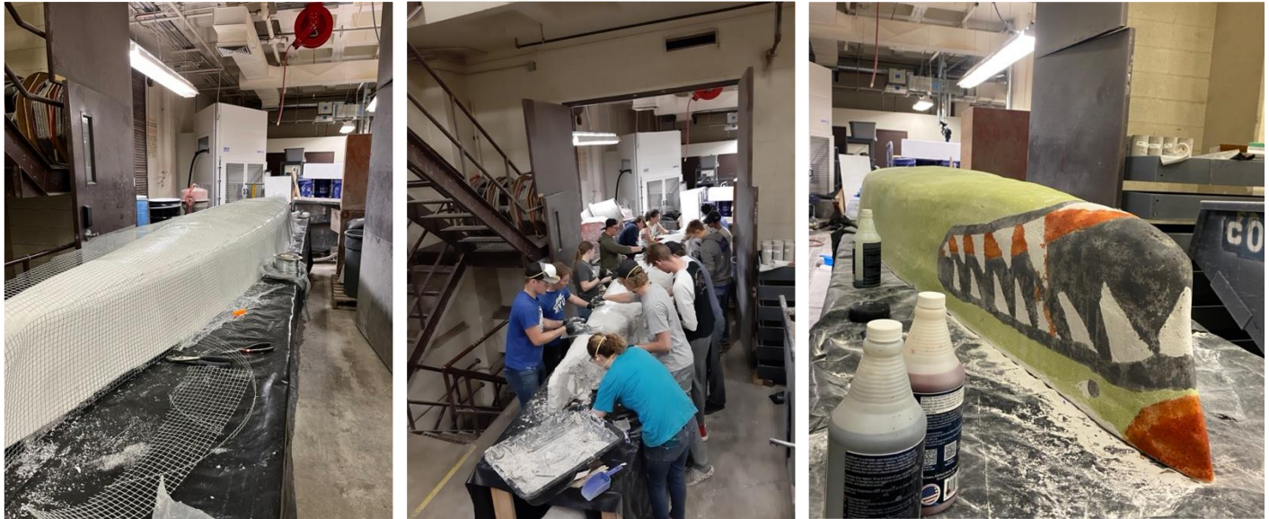
Figure 6: Assembling the Steel Reinforcement (left), Casting the Canoe (middle), Final Stained Canoe (right)
